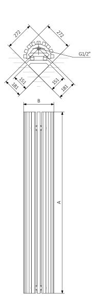
A - Height B - Width C1-C5 - Distance between pipe centres D - Horizontal distance between mounting bracket centres E - Vertical distance between mounting brackets F - Distance between a mounting bracket and the bottom of the radiator
