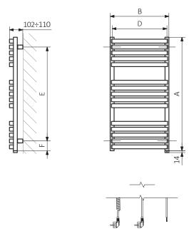
$A - Height \ B - Width \ C1-C5 - Distance \ between \ pipe \ centres \ D - Horizontal \ distance \ between \ mounting \ bracket \ centres \ E - Vertical \ distance \ between \ mounting \ brackets \ F - Distance \ between \ a \ mounting \ bracket \ and \ the \ bottom \ of \ the \ radiator$
