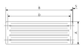
$A-Height \quad B-Width \quad C1-C5-Distance \ between \ pipe \ centres \quad D-Horizontal \ distance \ between \ mounting \ bracket \ centres \\ E-Vertical \ distance \ between \ mounting \ brackets \quad F-Distance \ between \ a \ mounting \ bracket \ and \ the \ bottom \ of \ the \ radiator$
