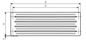
$A-Height \quad B-Width \quad C1-C5-Distance \ between \ pipe \ centres \quad D-Horizontal \ distance \ between \ mounting \ bracket \ centres \\ E-Vertical \ distance \ between \ mounting \ brackets \quad F-Distance \ between \ a \ mounting \ bracket \ and \ the \ bottom \ of \ the \ radiator$
